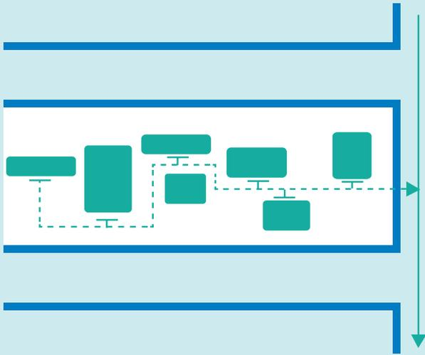
**Conventional sewerage:** each plot has a separate connection to the street sewer
