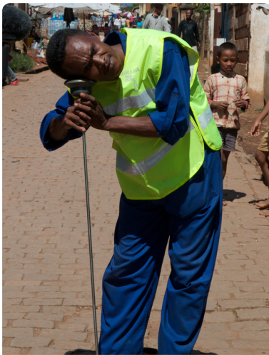
A member of JIRAMA's NRW Reduction Team uses a listening stick to detect leaks
